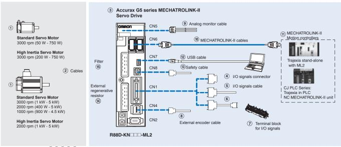
Note: The symbols ① ② ③ ④ ⑤... show the recommended sequence to select the components in Accurax G5 servo system
