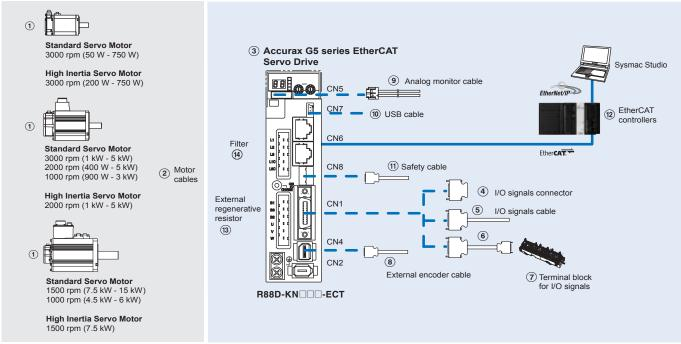
$\textbf{Note:} \ \ \textbf{The symbols} \ \ \textbf{\^{1}2345}... \ \ \textbf{show the recommended sequence to select the components in Accurax G5 servo system}$
