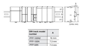
Consider the following points when expanding the configuration: - The total length of I/O connecting cable must not be exceed 12 m. - I/O Connecting cables require the bending radius indicates below. Note: 1.
