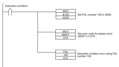
**Note** Use the same methods as for actual system errors to clear the simulated system errors. Refer to the *11-2 Troubleshooting* for details. All system errors simulated with FAL(006) and FALS(007) can be cleared by cycling the power supply.
