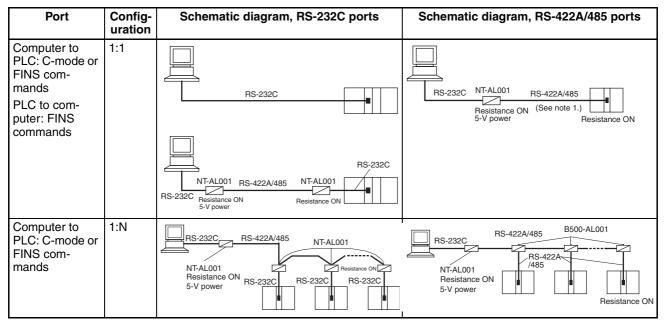
**Note** (1) Four-wire connections must be used for RS-422A/485 connections with Host Link communications.
