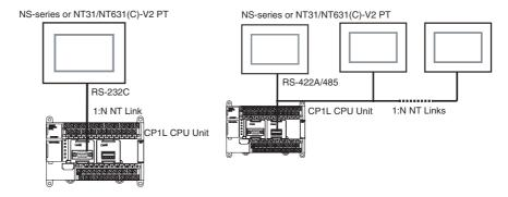
Note Communications are not possible using the 1:1-mode NT Link protocol.
