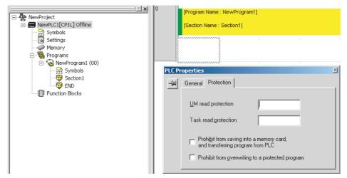
Connect online and select PLC - Transfer - To PLC to transfer the program. The tasks registered in step 2 will be password-protected.
