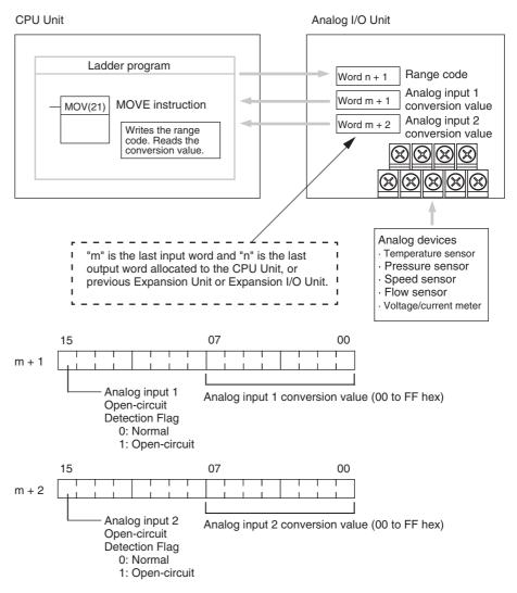
Note The Open-circuit Detection Flag is turned ON if the input signal range is set to 1 to 5 V or 4 to 20 mA and the input signal falls below 1 V or 4 mA. (Open circuits are not detected when the input signal range is set to 0 to 10 V.)
