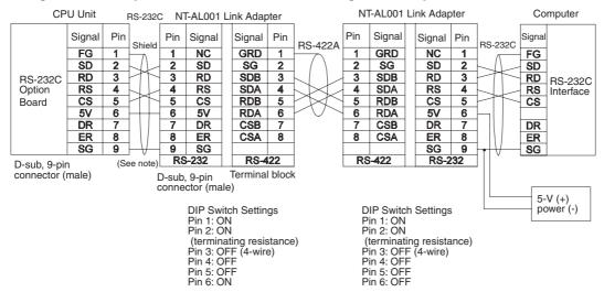
Note We recommend using the following NT-AL001 Link Adapter Connecting Cables to connect to NT-AL001
