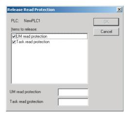
2. Input the password. If the password is incorrect, one of the following messages will be displayed and protection will not be released.
