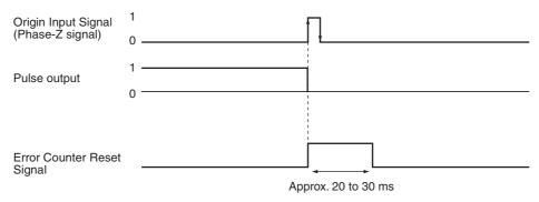
When the Origin Proximity Input Signal is received, the motor will begin decelerating from the origin search high speed to the origin search proximity speed. In this operating mode, the motor will stop at the Origin Input Signal after deceleration is completed.
