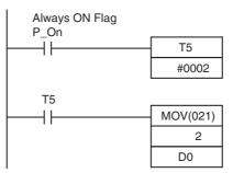
TIM 5 will start as soon as power turns ON. After 0.1 to 0.2 s (100 to 200 ms), the input for TIM 5 will turn ON, and the converted data from analog input 0 that is stored in word 2 will be transferred to D00000.
