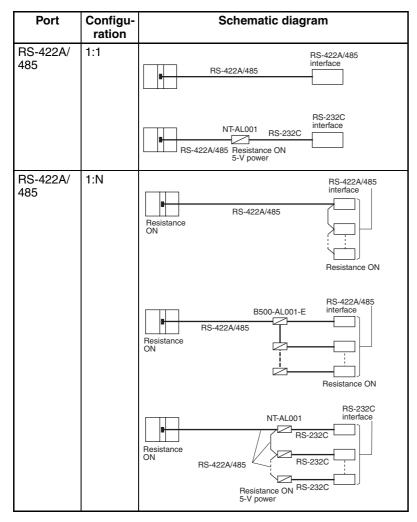
**Note** (1) The maximum cable length for RS-232C is 15 m. The RS-232C standard, however, does not cover baud rates above 19.2 Kbps. Refer to the manual for the device being connected to confirm support.
