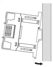
3. Press in all of the DIN Track mounting pins to securely lock the Units in place.
