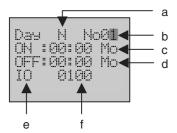
Press the **OK** button to enter the Day Timer Screen. The final digit of the Timer No. will be flashing. The following table shows the setting items.
