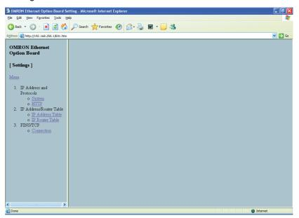
4. Select 1. IP address and Protocols - System to display System menu.
