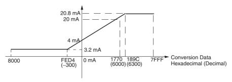
Averaging Function for Analog Inputs The averaging function can be enabled for inputs using the DIP switch. The averaging function stores the average (a moving average) of the last eight input values as the converted value. Use this function to smooth inputs that vary at a short interval.
