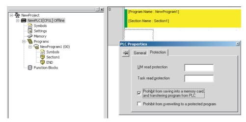
2. Go online and then either select *PLC - Transfer - To PLC* to transfer the program or select *PLC - Protection - Set Password* and click the **OK** button.
