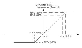
Voltage in the 0 to 10 V range corresponds to hexadecimal values 0000 to 1770 (0 to 6,000). The range of data that can be converted is FED4 to 189C hex (-300 to 6,300). A negative voltage is expressed as two's complement.
