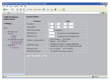
5. Make the required settings (i.e., the IP address in this example).
