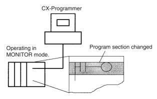
The cycle time will be increased by from one to several cycle times if the program in the CPU Unit is edited online in MONITOR mode. The cycle time will also be increased to back up data in the flash memory after online editing. The BKUP indicator will be lit during this period and the progress of the backup will be displayed on the CX-Programmer. The increases per cycle are listed in the following table.
