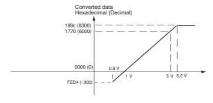
Voltage in the 1 to 5 V range corresponds to hexadecimal values 0000 to 1770 (0 to 6,000). The range of data that can be converted is FED4 to 189C hex (-300 to 6,300). Voltage in the range of 0.8 to 1 V is expressed as two's complement.
