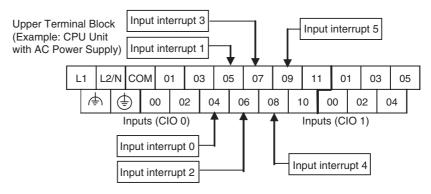
Input Terminal Block of CPU Units with 40 I/O Points
