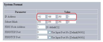
> 6. After entering the correct values, click the Transfer Button to transfer the settings to the Ethernet Option Board.
