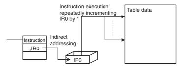
The Index operation uses the following procedure.
