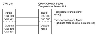
In this example, 100 times the temperature data for temperature input 0 is stored in binary form in D100 to D102.
