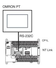
With the NT Link protocol, the PLC automatically responds to commands sent from the PT, so no communications programming is required in the CP1L.
