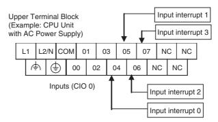
Input Terminal Block of CPU Units with 20 I/O Points
