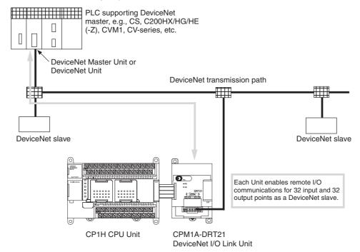
From the standpoint of the CP1L CPU Unit, the 32 input bits and 32 output bits allocated to the DeviceNet I/O Link Unit are identical to input and output bits allocated to Expansion I/O Units even though the DeviceNet I/O Link Unit does not control external inputs and outputs. The input and output bits allocated to the DeviceNet I/O Link Unit are one side of an I/O link between the slave CPU Unit and the CP1L CPU Unit to which the Master Unit is connected.
