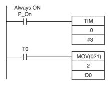
TIM 0 will start as soon as power turns ON. After 0.2 to 0.3 s (200 to 300 ms), the input for TIM 0 will turn ON, and the converted data from analog input 0 that is stored in word 2 will be transferred to D00000.
