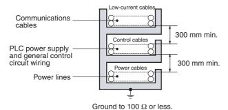
• If the I/O wiring and power cables must be placed in the same duct, they must be shielded from each other using grounded steel sheet metal.
