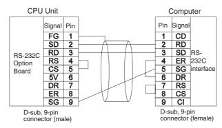
Using NT-AL001 Converting Link Adapters
