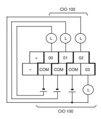
AC-power-supply models have a 24-VDC output terminals (+/-) on the lower terminal block. They can be used as a DC power supply for the input circuit.
