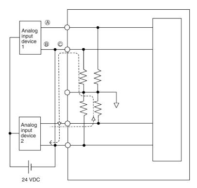
For example, if analog input device 2 is outputting 5 V and the same power supply is being used as shown above, about 1/3, or 1.6 V, will be applied at the input for input device 1.
