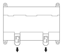
2. Lower the Units so that they catch on the top of the DIN Track, and then press them forward all the way to the DIN Track at the bottom.
