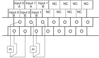
Temperature input 0 Temperature input 1
