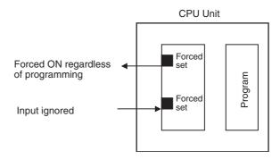
The following areas can be force-set and reset: CIO Area, Work Area, Timer Completion Flags, HR Area, Counter Completion Flags.
