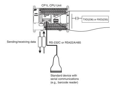
For example, simple (non-protocol) communications can be used to input data from a barcode reader or output data to a printer.
