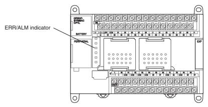
When the ERR/ALM indicator flashes, connect the CX-Programmer to the peripheral port and read the error messages. If a low battery message appears on the CX-Programmer (see note 1) and the Battery Error Flag (A402.04) is ON (see note 1), first check whether the battery is properly connected to the CPU Unit. If the battery is properly connected, replace the battery as soon as possible.
