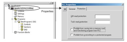
2. Go online and then either select *PLC - Transfer - To PLC* to transfer the program or select *PLC - Protection - Set Password* and click the **OK** button.
