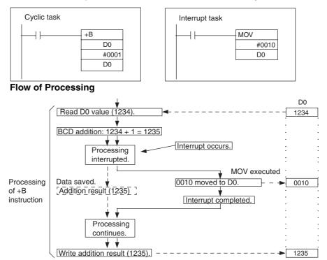
The interrupt occurs during processing of the +B instruction and the result is saved temporarily without being written to the destination word (D0).
