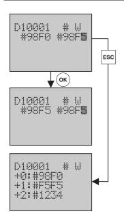
3. Use the **Forward** button to move the column cursor to the data of I/O memory. Use the **Down** or **Up** button to change the value of each digit.
